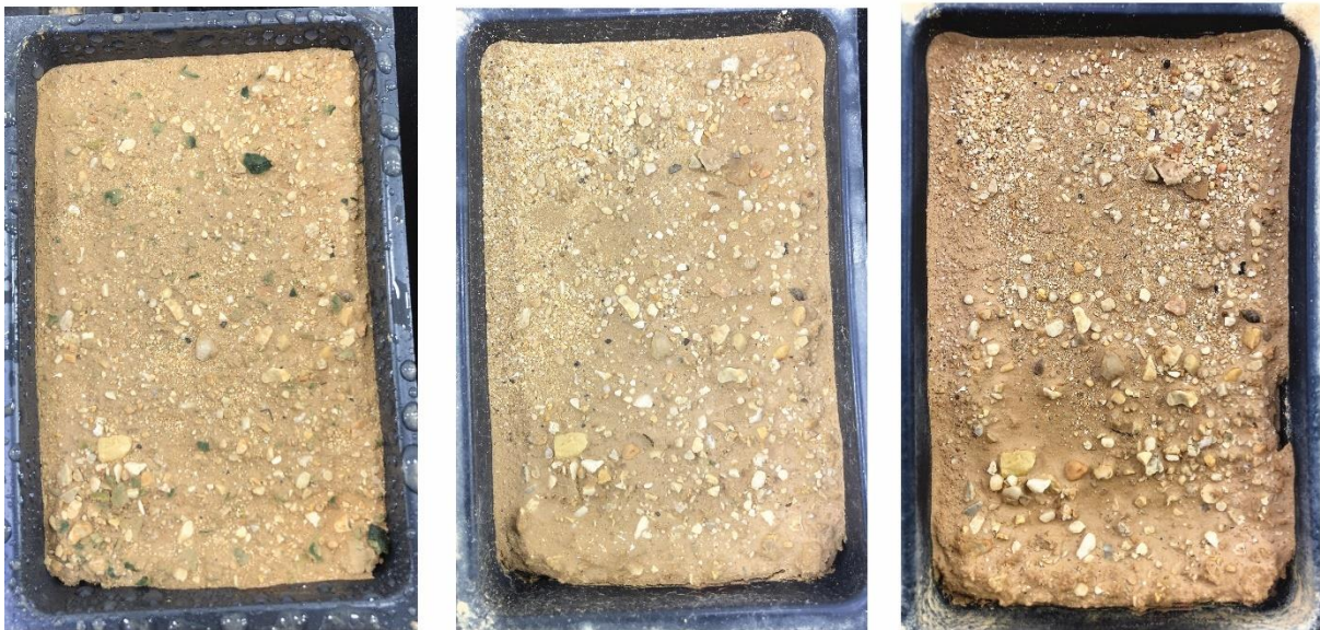
Figure 15. Pictures taken during the experiment. (a) examples of salt accumulation on the soil surface. (b) An example of disappearance of green pigment in a sample inoculated with cyanobacteria enriched biocrusts, after the first hydration event (left), 10 hydration events (middle) and 20 hydration events (right).
