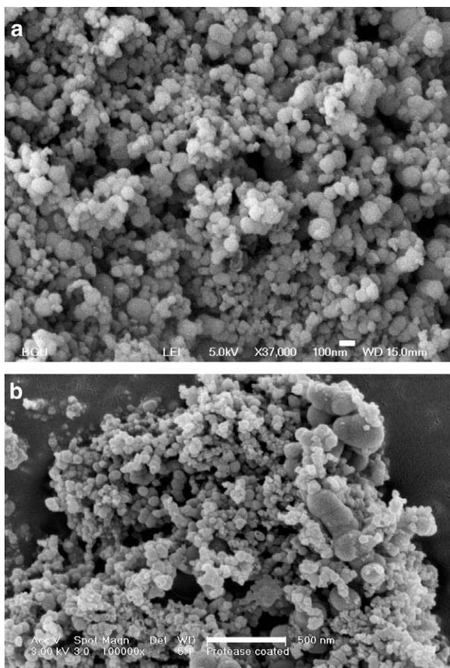
**Fig. 3.** SEM micrographs of synthetic ACC. (a) ACC comprising 50–250 nm nanospheres produced with the addition of *ISM-total* (bar = 100 nm). (b) ACC comprising 50–250 nm nanospheres produced with *ISM-peptides* extracted by proteases (bar = 500 nm).
