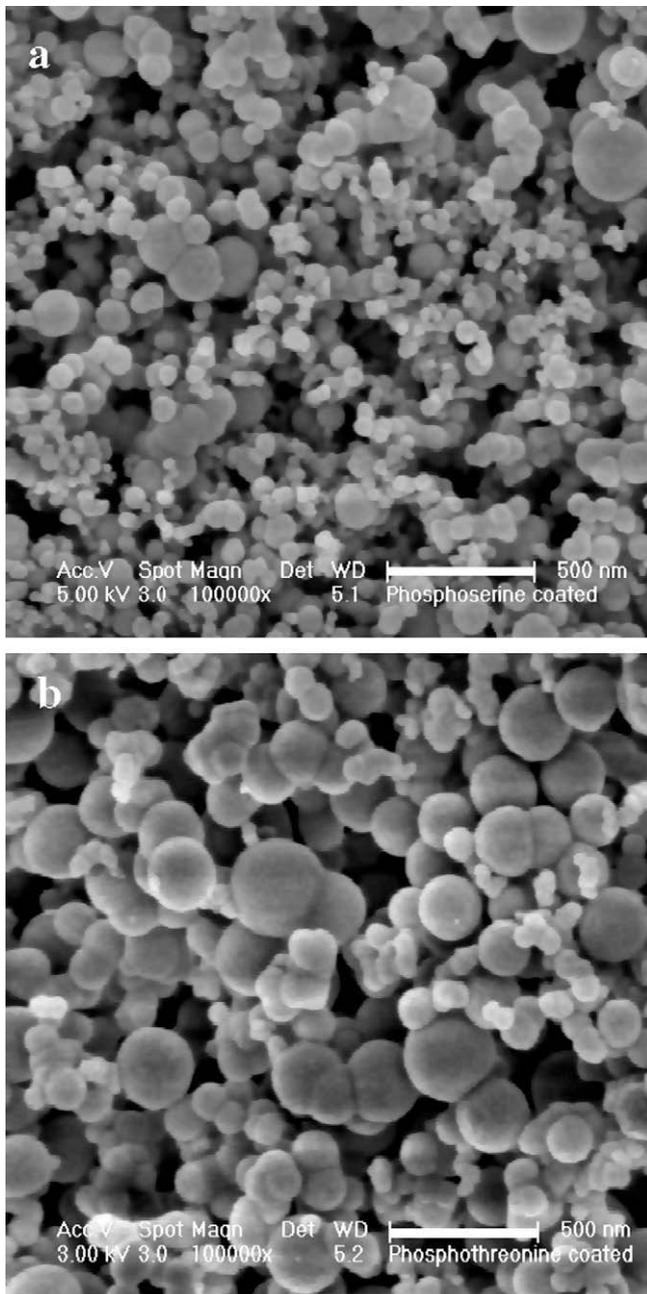
**Fig. 7.** (a) SEM micrographs of ACC produced in the presence of P-Ser comprising 20-nm to 200-nm nanospheres (bar = 500 nm). (b) ACC induced by P-Thr (1 mM), composed of 50-nm to 300-nm nanospheres (bar = 500 nm).
