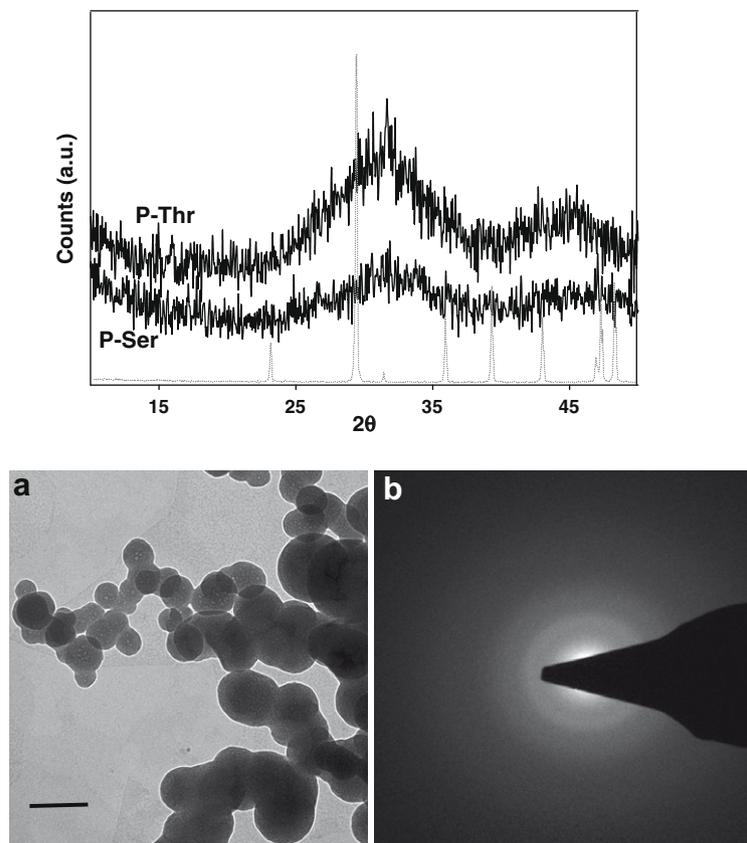
**Fig. 8.** X-ray and electron diffraction of synthetic ACC. (a) XRD diffractogram of ACC precipitated in the presence of 2 mM P-Ser and in the presence of 1 mM P-Thr; diffractogram of calcite is shown in gray. (b) TEM image of ACC produced in the presence of P-Thr (bar = 200 nm). (c) Selected area electron diffraction acquired from this region, demonstrates the amorphous nature of the precipitate.
